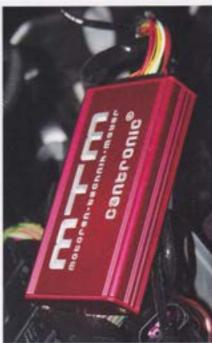
Of course, Barry preferred to let QST take care of the installation and a subsequent performance test on the in-house Maha LPS 3000 PKW fourwheel-drive chassis dyno revealed the full extent of the improvement. Maximum power output is now 433 PS, an improvement of exactly 100 PS on that of the standard engine, and it is produced over a similarly wide range a plateau rather than a peak — between 5800 and 7000 rpm, with the actual ultimate figure occurring at 6600 rpm.
